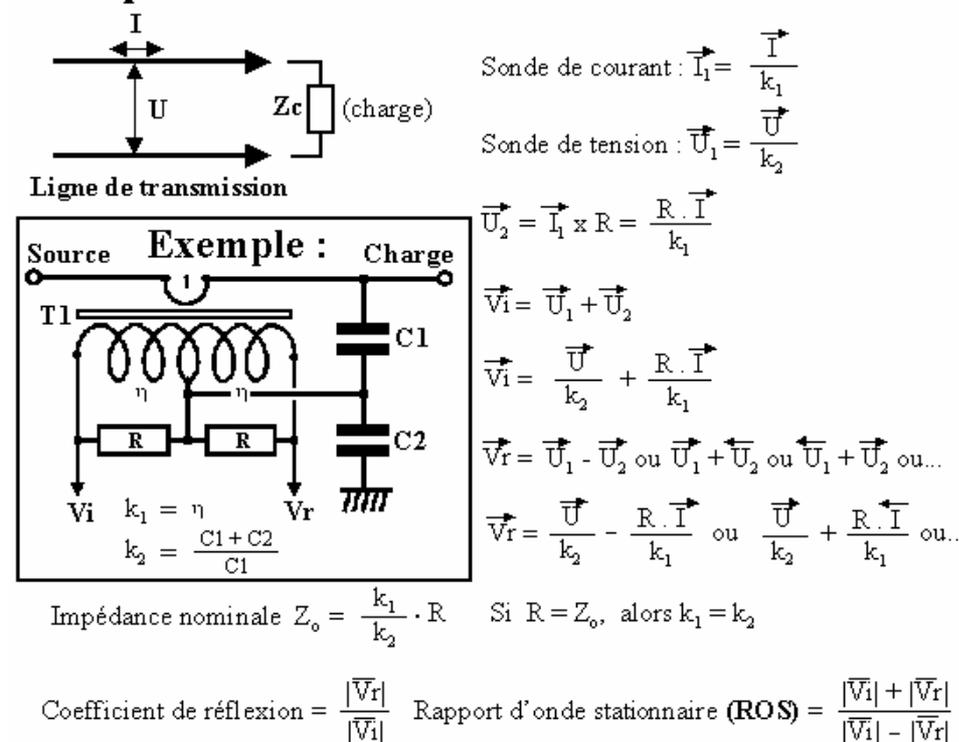
$$\text{Puissance transmise} = K \times (V_i^2 - V_r^2) = U \times I \times \cos(\varphi)$$
