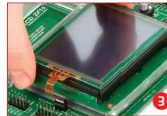
Figure 13-3: Now place GLCD with Touch panel into GLCD socket
