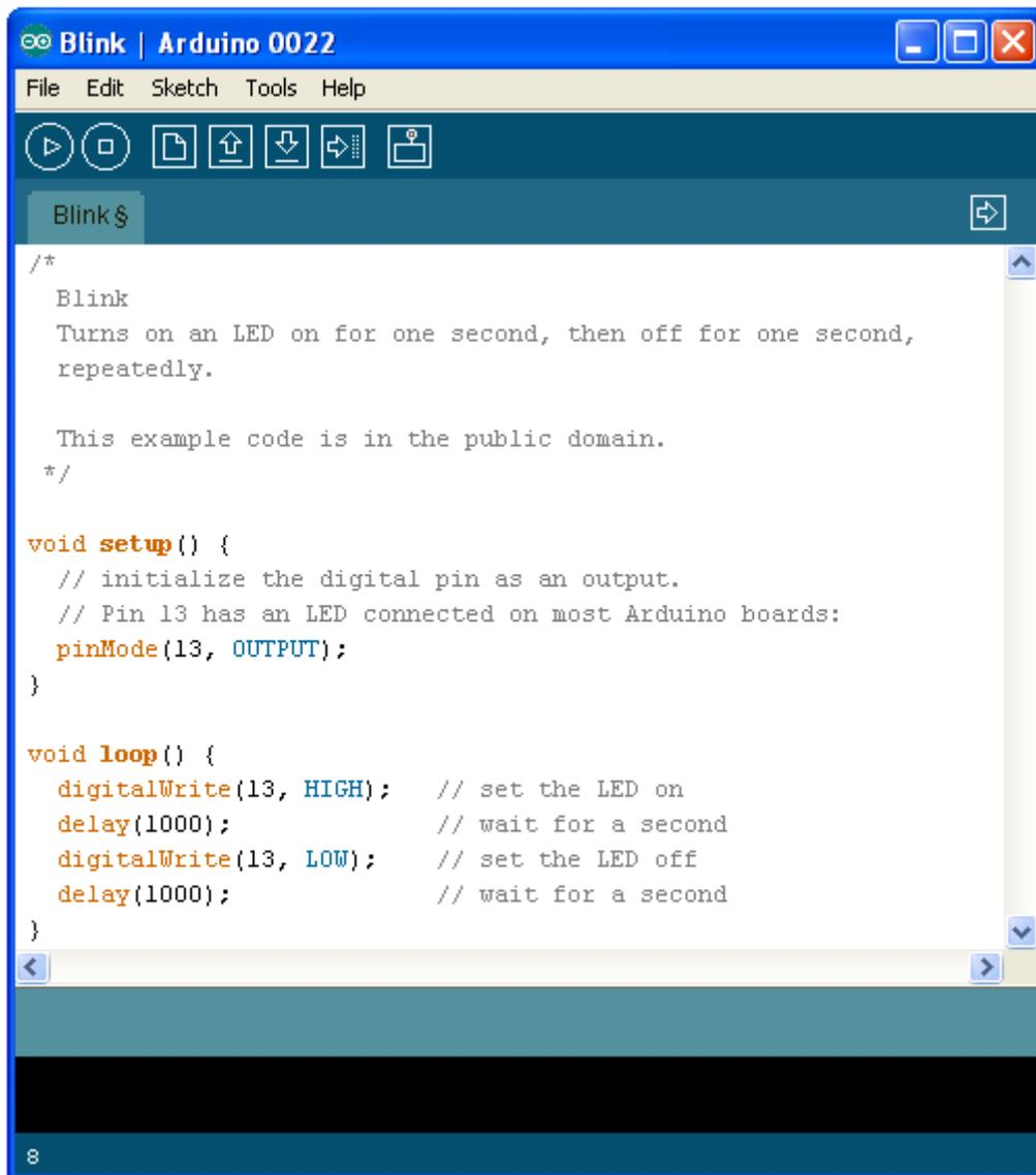
The screenshot shows the Arduino IDE interface. The title bar reads "Blink | Arduino 0022". The menu bar includes "File", "Edit", "Sketch", "Tools", and "Help". Below the menu bar is a toolbar with icons for running, stopping, saving, uploading, downloading, and refreshing. The main text area contains the following code:
