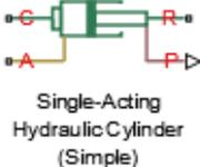
Single-Acting Hydraulic Cylinder (Simple) | Simscape/SimHydraulics/Hydraulic Cylinders                   |
