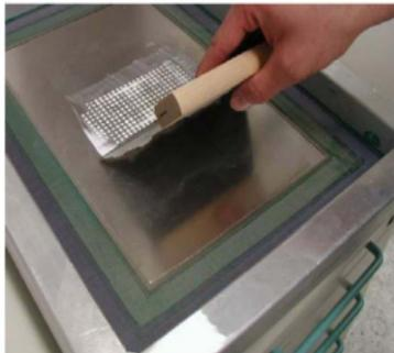
Fig. 5: Blade squeezing
