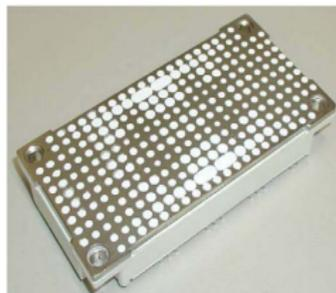
Fig. 6: Print image after blade squeezing
