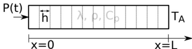
$$hS\rho C_p \frac{\partial T_i(t)}{\partial t} = \lambda S \frac{T_{i+1}(t) - T_i(t)}{h} - \lambda S \frac{T_i(t) - T_{i-1}(t)}{h}$$
